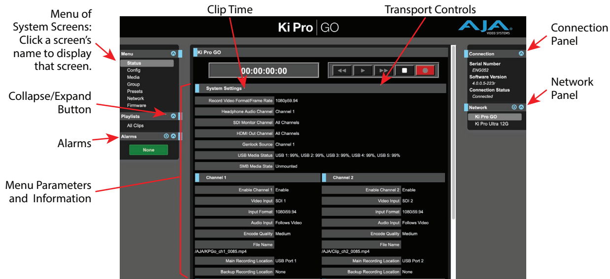
Figure 19. Ki Pro GO Web UI Status Screen Example
