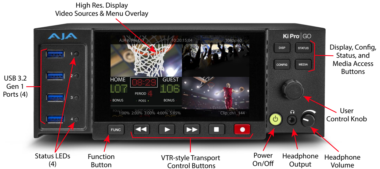
Figure 2. Ki Pro GO Front Panel
