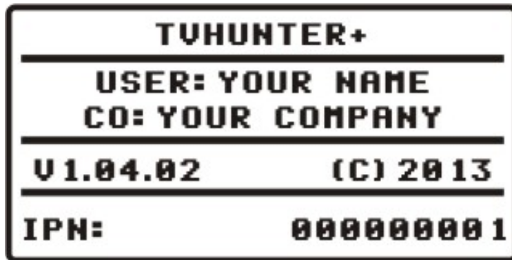
Figure 3. Name of the instrument (TVHUNTER+), user's name, company, firmware's version (v1.04.02), year and serial number.
