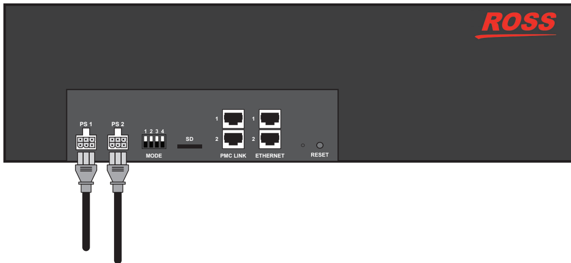
Figure 3.4 MC1-PANEL-16 — Power Connections
